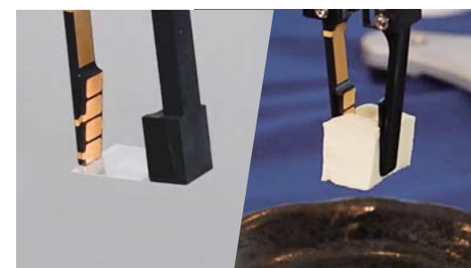
MoR® picking up a microscope slide and a piece of soft tofu
